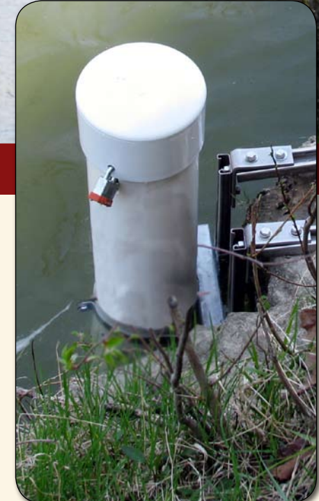
This special assembly houses a SDL500 Data Logger and protects against vandalism.
