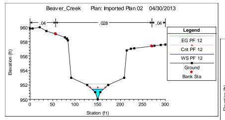
• Stage height at Vnotch is 1.43 ft.  Stage height of crosssection following Vnotch is 1.94 ft.
