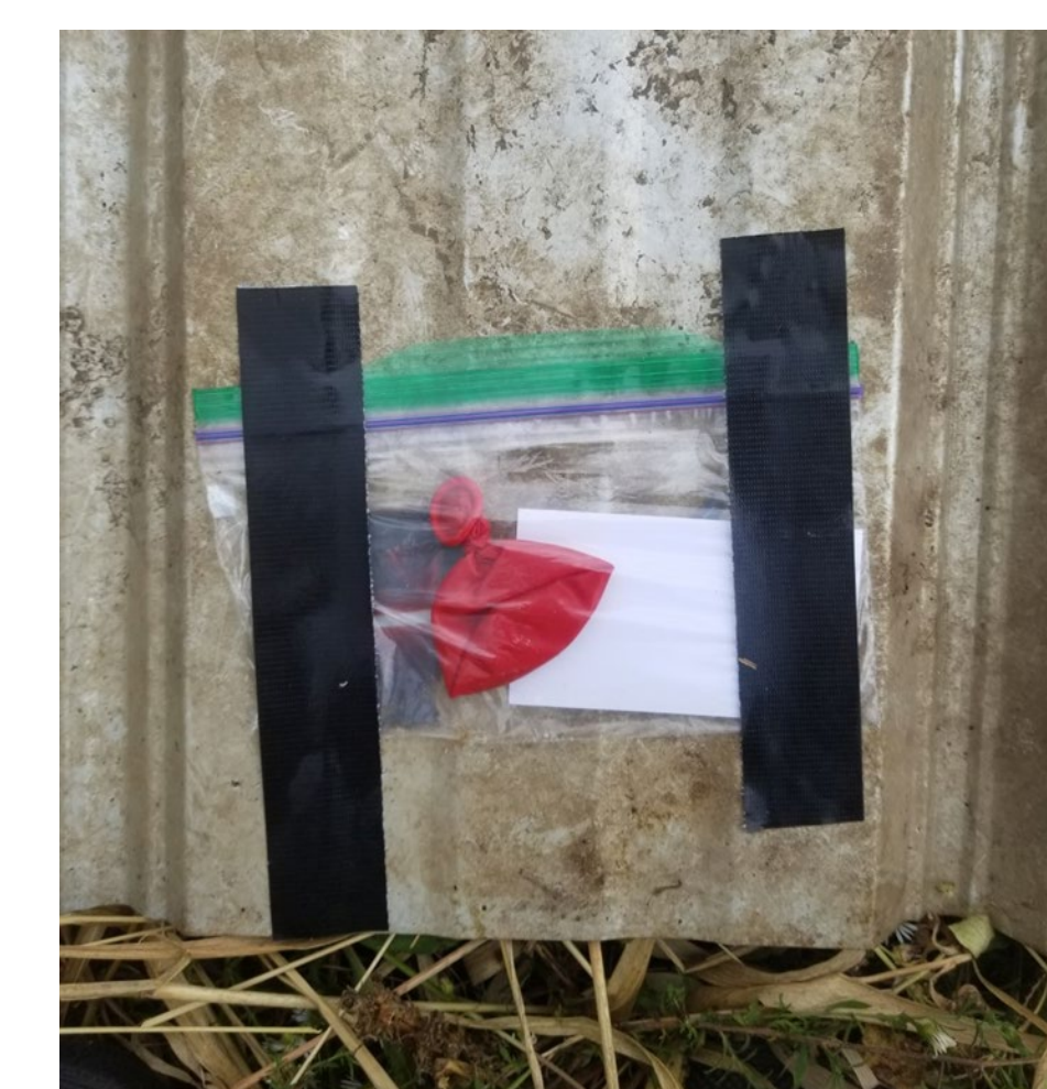
Photo 1: Tin Coverboard temperature logger placed into a Ziplock bag and taped to the underside of a tin coverboard to record tin temperature.
