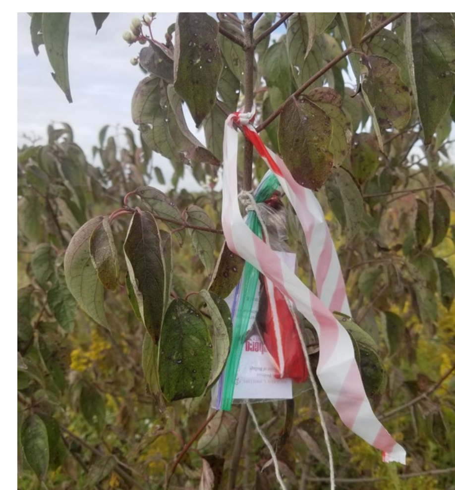
Photo 2: Ambient temperature logger placed into a Ziplock bag and tied into a small tree with flagging to easily find and record ambient temperature.
